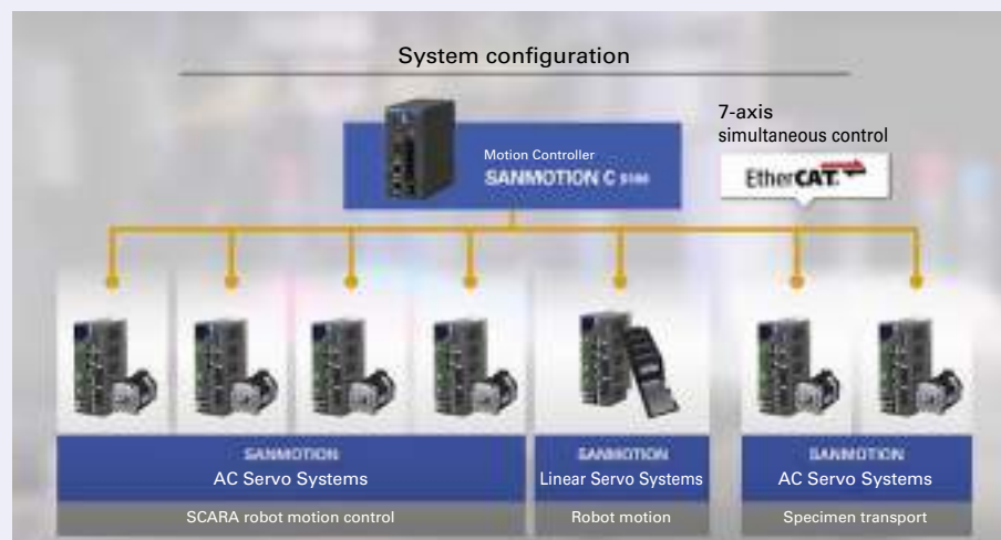
Comprehensive solution example: SCARA robot control demo
