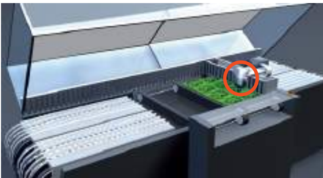
SuperShorty sensors in electronics production: SMT placement equipment
