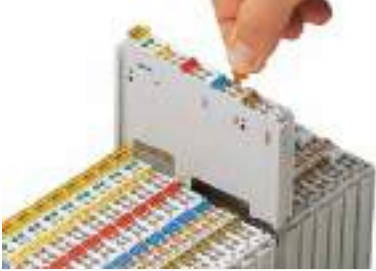
Securing/removing a module from the DIN-rail
