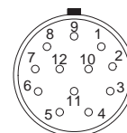
Counting direction cw (e.g. female connector)
