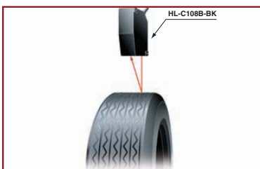
Inspecting tire form
