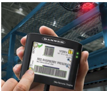
RD35 Handheld Remote Display Used for- programming
